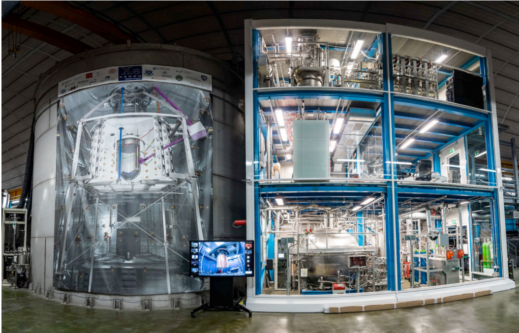
Figure 2.1: XENONnT experiment with the water tank (left), cooling and purification systems and data read-out infrastructure (right) located underground. Image credit: XENON collaboration.
