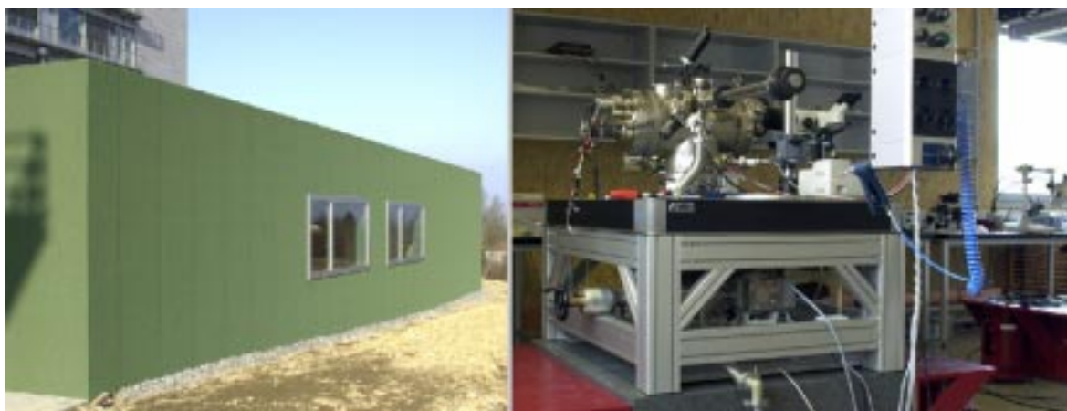
Figure 13.1: At left, a view of the new laboratory building is shown. At right, the Low Energy Electron Point Source (LEEPS) microscope, mounted on a vibration damping stage, is shown. A total of four such platforms are available inside the new building. They are embedded in three orthogonal Helmholtz coil pairs used for compensating the local magnetic field to protect the coherence of our low energy electrons.
