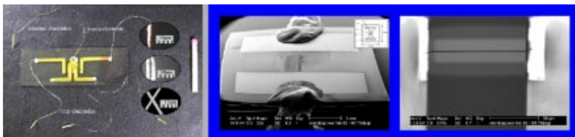
Figure 13.3: Left: "Home-made" simple device for manipulating DNA molecules in liquids [1]. Right: Integrated chip structure, fabricated by Clondiag Chip Technologies.
