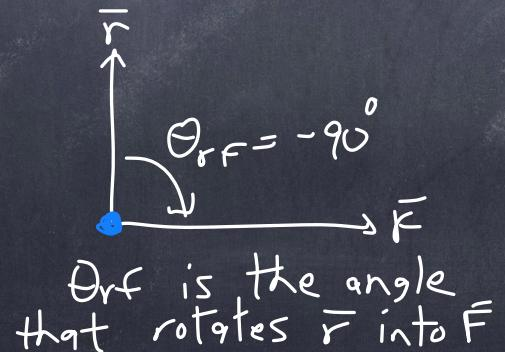
$\theta_{rf}$  is the angle that rotates  $\bar{r}$  into  $\bar{F}$
