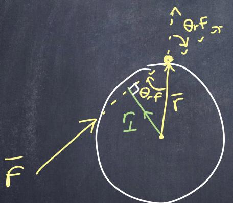
$r_{\perp}$ : component of  $\vec{r}$  that is  $\perp$  to  $\vec{F}$
