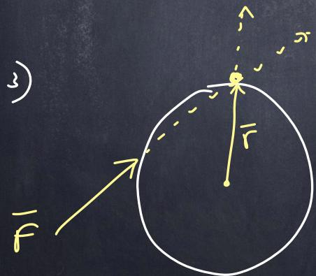
Torque can be also thought of as the product of the force with the "lever arm"  $= r_{\perp} =$  the part or component of  $\vec{r}$  that is perpendicular to the force.
