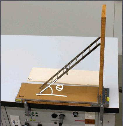
What is the smallest angle,  $\Theta_{\min}$ , such that the ladder does not fall?
