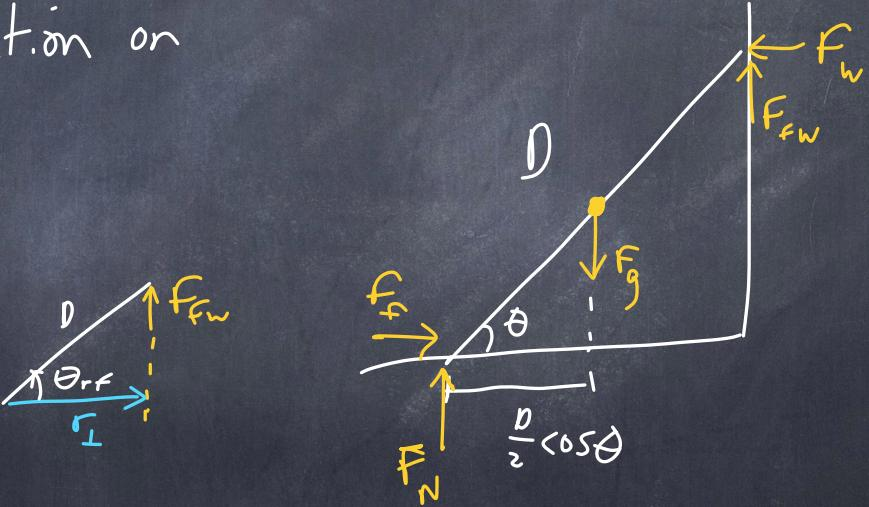
$$T_{ccw} = r_{\perp} F_{fw} = (D \cos \theta) F_{fw}$$
