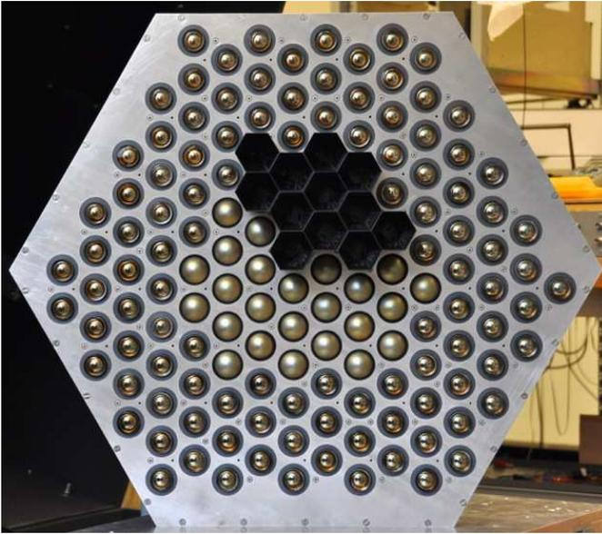
FIG. 7.3 – The 144-pixel prototype photon detector.
