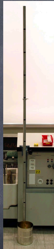
dropping magnet in a conductor
