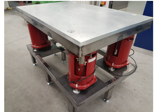
The three photograph are examples for work done in our workshop: prototype of the DARWIN Demonstrator for the group Baudis (left), a digitizer for old films for the department of film studies UZH (middle) and a vibration damping table for the group Natterer (right).
