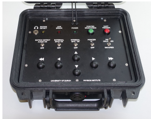
Case with the control electronics for an anaesthetic gun.
