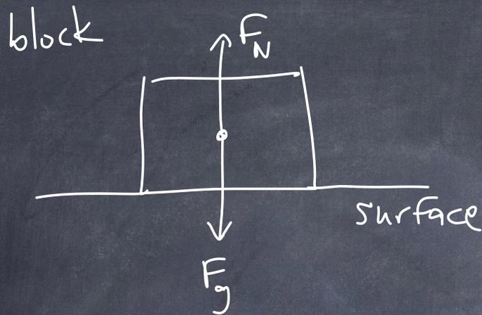
$F_N$ : normal force pushing on the block by the surface.
