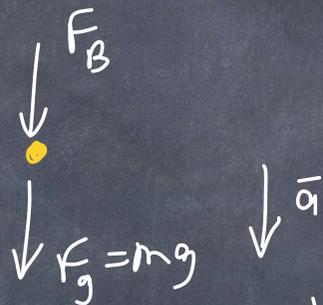
we want to solve for the case when the velocity is so slow ( $v_{\min}$ ) that the water is weightless  $\Rightarrow$  the bucket doesn't push into the water,  $F_B = 0$
