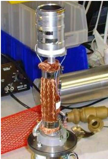
Figure 3.4: Our n-type HPGe detector before tests in liquid argon.
