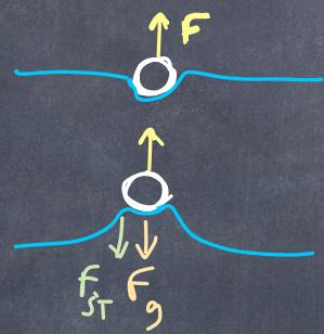
In this case, the surface tension resists us pulling the needle up, because we are stretching the membrane upward.
