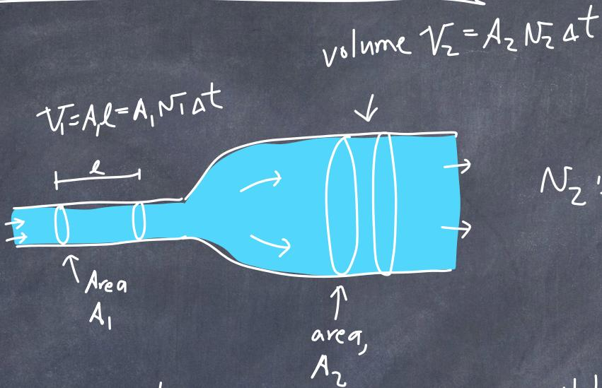
Since fluids are incompressible,  $V_1 = V_2$
