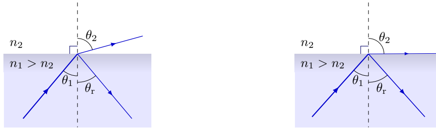
(a) Refraction angle \theta_2 quickly approaches 90^\circ . (b) When \theta_1 = \theta_c , the light is reflected totally.
