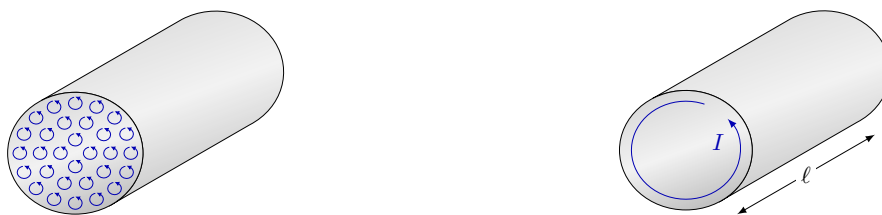
(a) Each atom has its own small current loops, and their own magnetic moment. (b) One can think of the microscopic currents adding up to one big one.
