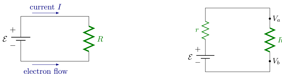
(a) Simple circuit with an EMF creating a potential \mathcal{E} and a resistor R .
