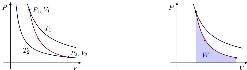
(a) Adiabatic expansion (red) between two isotherms. (b) Work done by an adiabatic expansion (red).
