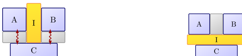
(a) A and B are each in thermal contact with C through conductors, but isolated from each other by insulator I. (b) A and B are each in thermal contact, but both isolated from C by I.
