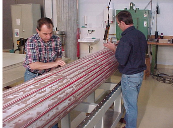
Figure 15.2: The grooves for the cables transmitting the cathode signals to the end flanges are filled with glue.
