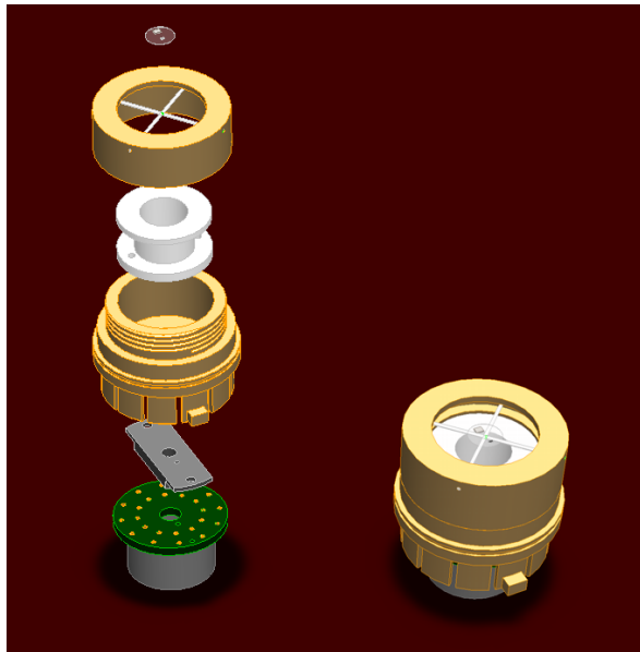
Figure 12.7: AC calorimeter puck that fits into a commercial PPMS (Quantum Design Inc.) system.
