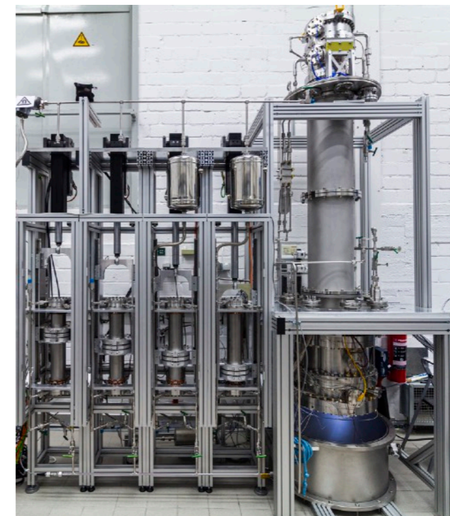
Rn distillation column for XENONnT (reduce ^{222}\text{Rn} - hence also ^{214}\text{Bi} - from pipes, cables, cryogenic system)
