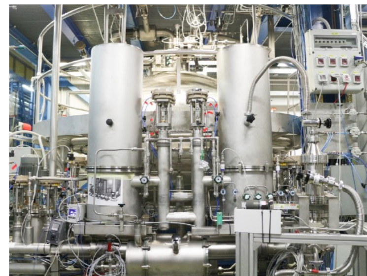
LXe purification system (5 L/min LXe, faster cleaning; 2500 slpm) for XENONnT
