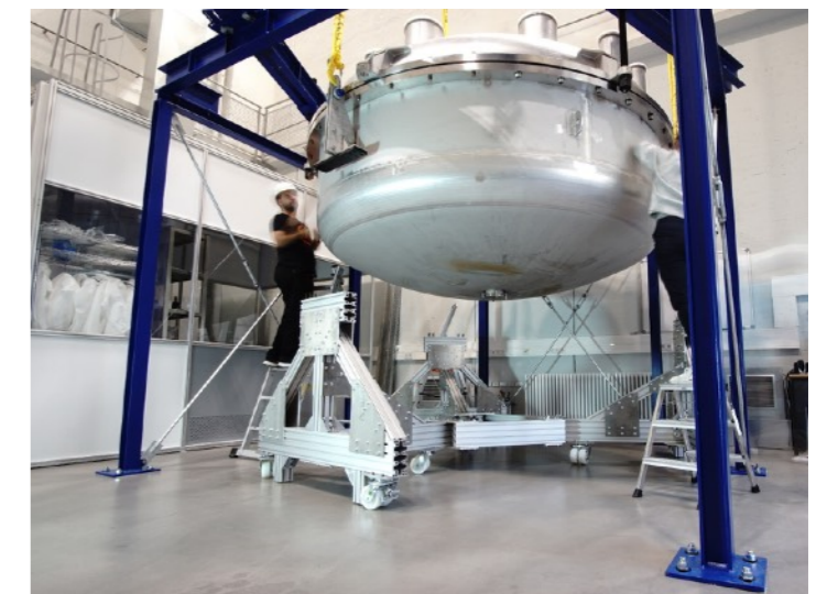
2.6 m diameter Xe TPC demonstrator for DARWIN
