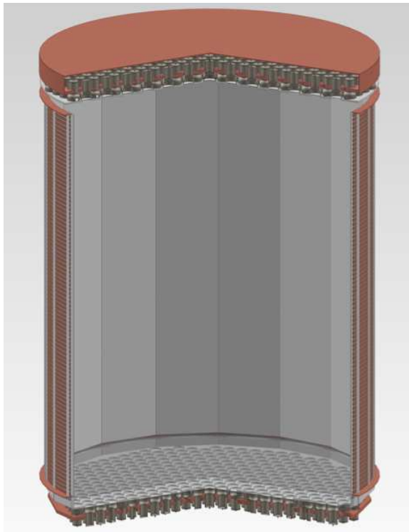
FIG. 5.1 – A CAD model of the 20 t LXe DARWIN TPC.
