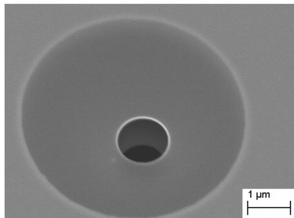
Figure 13.7: SEM image of a micro-lens taken at a tilt angle of  $30^\circ$ . The 5 micron bore covered on each side by a thin carbon flake is still visible.
