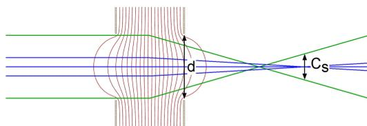
Figure 13.4: Schematic to illustrate the implication of lens dimensions  $d$  on the intrinsic spherical aberration  $C_s$  creating a disk of least confusion in the Gaussian focal plane of an electron lens.
