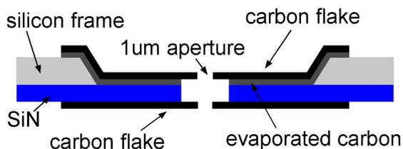
Figure 13.6: Schematic side-view of a micro lens.
