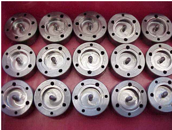
Figure 12.10: Probe holders made out of Molybdenum.
