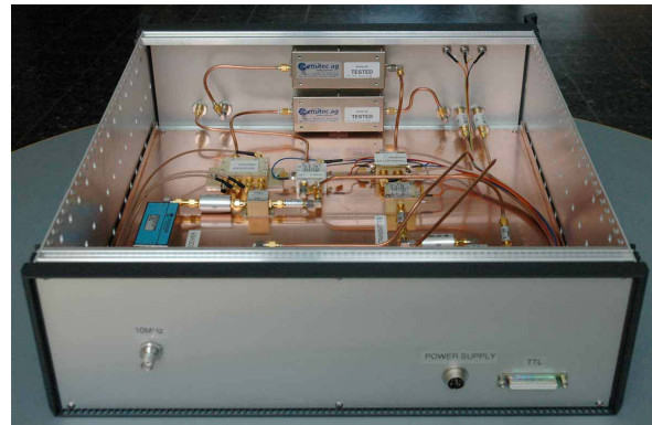
Figure 13.2: The SCOPES 70 MHz NMR-spectrometer high frequency device.
