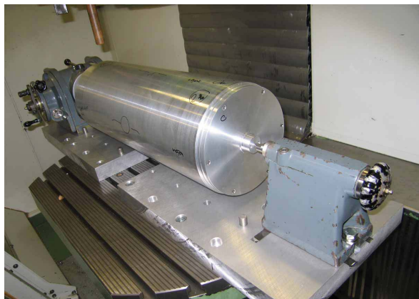
Figure 12.7: Mounting tool for the third detector layer.
