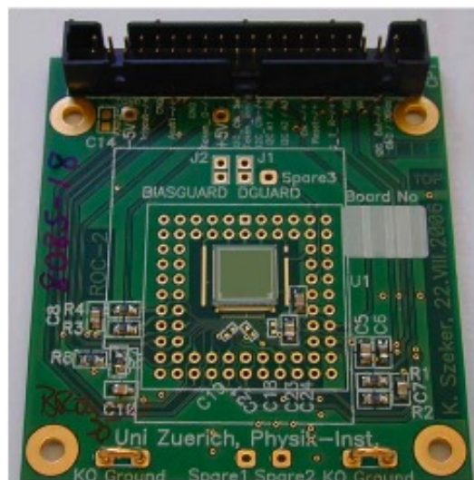
Figure 7.7: PCB housing a pixel sensor bump-bonded to the ROC.
