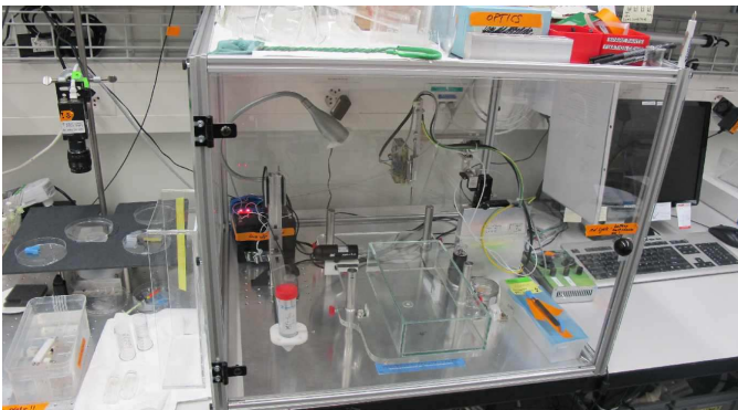
FIG. 17.7 – Top: Full setup, in the centre the fish channel with the laser camera is visible. Middle: Laser camera system. Bottom: Protective housing.
