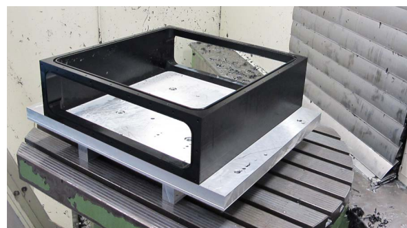
Fig. 17.9 – Housing of the Wilson chamber during machining on the mill.
