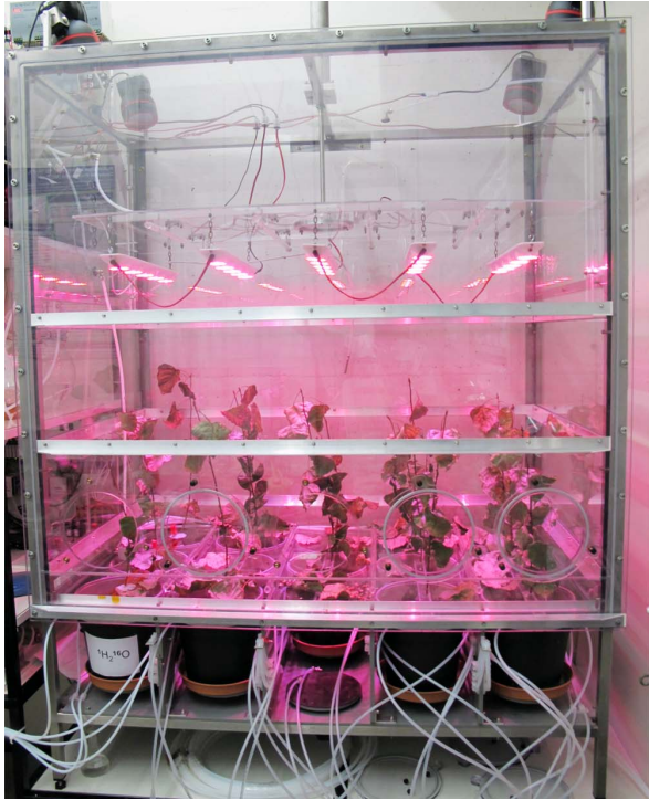
Fig. 17.11 – Sealed greenhouse with integrated control adaptors to study CO_2 metabolism.
