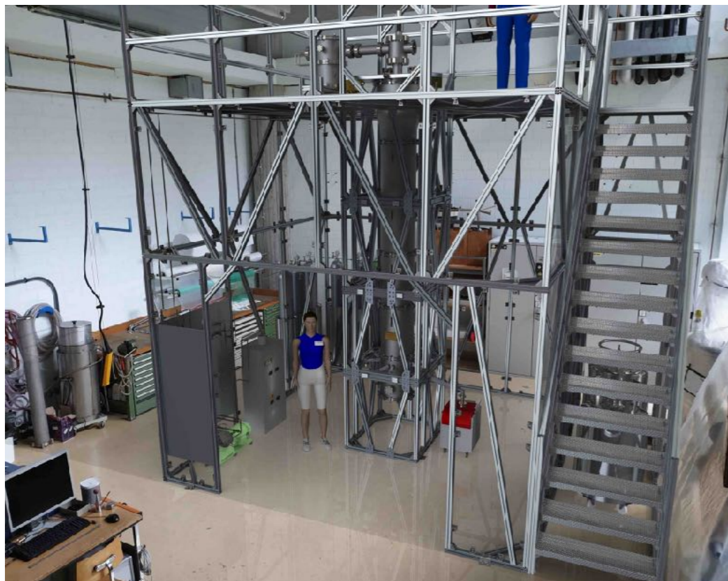
Test e^- drift over 2.6 m (purification, high-voltage)
