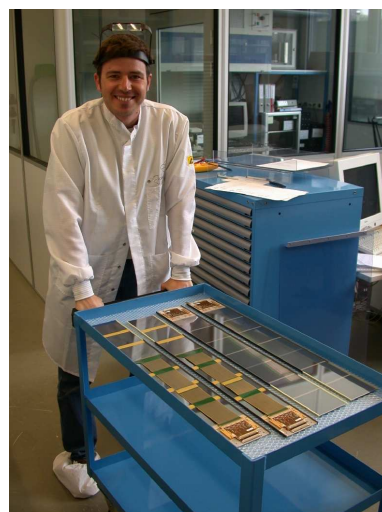
Figure 7.6: Two stage-I modules and two completed modules on their way from the production lab to the burn-in test stand.
