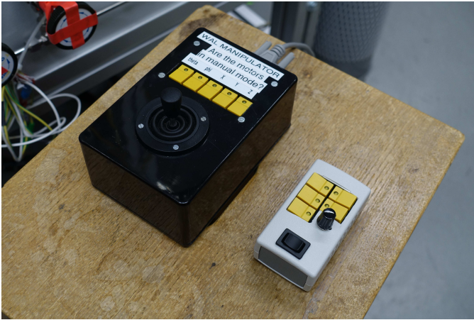
FIG. 16.3 – New remote control for the WALKUERE manipulator next to its old and larger version.
