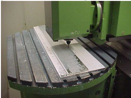
Figure 12.5: Support plate for the production of the cooling balconies of the LHCb inner tracker. Eight pieces are machined in parallel.
