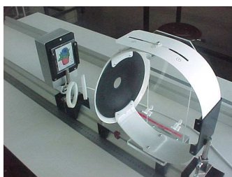
Optical bench with the model of the human eye. The focal distance is adjustable.
