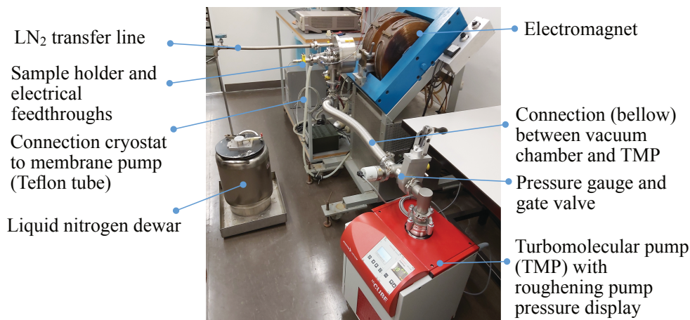
Figure 5: The vacuum system used in this experiment. The dewar of a former cryopump is used as storage vessel for liquid nitrogen. The cooling agent is pumped through the transfer line into and out of the cryostat by means of a small membrane pump (not on the picture). The nitrogen flow is controlled by a valve installed close to the computer screen.
